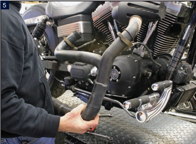
5 Remove the exhaust system from the bike and use a vice or some other method to hold the pipes secure without damaging them.
