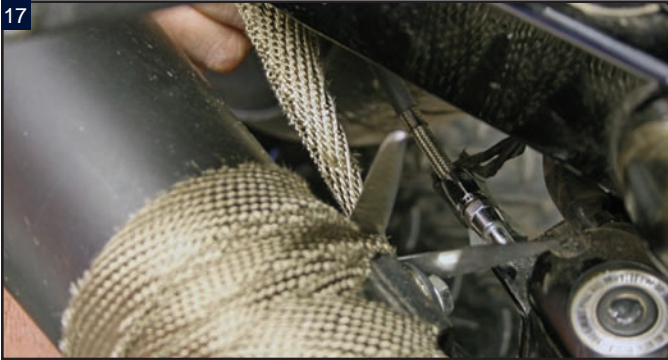
Secure the wrap by doubling it over itself and use a locking tie to hold it in place. Cut off any excess wrap.
