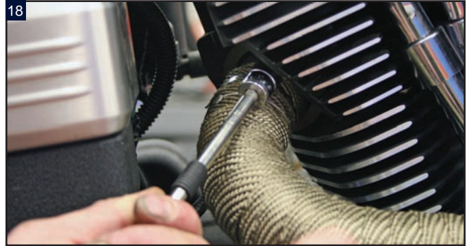
Tighten the head bolts on the rear cylinder.
